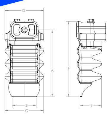
NOTE: For tools with standard hubs, effective tool height is reduced by 6.6mm compared to Traditional Fingers
